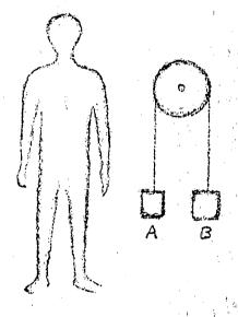
By imagining the outline of the human being we may arrive at the following concept. Let us assume that the person in the diagram is lifting a weight by hand, in our case a heavy object weighing one kilogram. The object is lifted by hand. Let us now ignore the person and, instead, tie the object (A) to a rope, pass the rope over a pulley, and tie another object of either identical or heavier weight to the other end (B). If B happens
